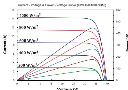
\* The specifications are obtained under the standard test conditions: 1000W/m<sup>2</sup> solar irradiance, 1.5 Air Mass and cell temperature of 25°C. Measurement uncertainty for all panels is 3%. The actual transactions will be subject to the contracts. These parameters are for reference only and it is not a part of the contracts. The technical specifications in this document may vary. For more information, refer to the "Installation Manual".
